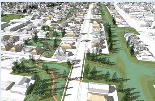
Spaces for water are integrated into streets and vacant lots Image: NORA, CDM Smith
